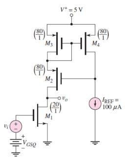
5. (20%) The parameters of the transistors are  $V_{TN} = 0.8 \text{ V}$ ,  $V_{TP} = -0.8 \text{ V}$ ,  $k'_n = 100\mu\text{A/V}^2$ ,  $k'_p = 60\mu\text{A/V}^2$ , and  $\lambda_n = \lambda_p = 0$ . The transistor (W/L) ratios are given in the figure. For  $R = 100 \text{ k}\Omega$ , determine (a)  $I_{REF}$ , (b)  $I_1$ ,  $I_2$ ,  $I_3$ , and  $I_4$ .
