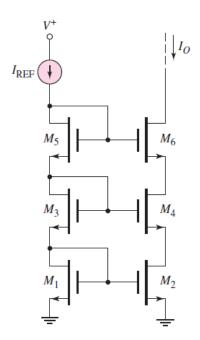
4. (25%) The parameters of the transistors are  $V_{TN} = 0.6 \text{ V}$ ,  $V_{TP} = -0.6 \text{ V}$ ,  $k'_n = 100\mu\text{A/V}^2$ ,  $k'_p = 60\mu\text{A/V}^2$ , and  $\lambda_n = \lambda_p = 0.02\text{V}^{-1}$ . The width-to-length ratios are shown in the figure. The value of  $V_{GSQ}$  is such that  $I_{D1} = 100\mu\text{A}$ , and  $M_1$  and  $M_2$  are biased in the saturation region. Determine the small-signal voltage gain  $A_v = v_o/v_i$ .
