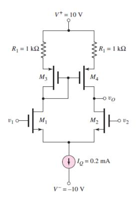
**4.** (25%) The bias currents  $I_1$  and  $I_2$  are such that a zero dc output voltage is established. The transistor parameters are:
