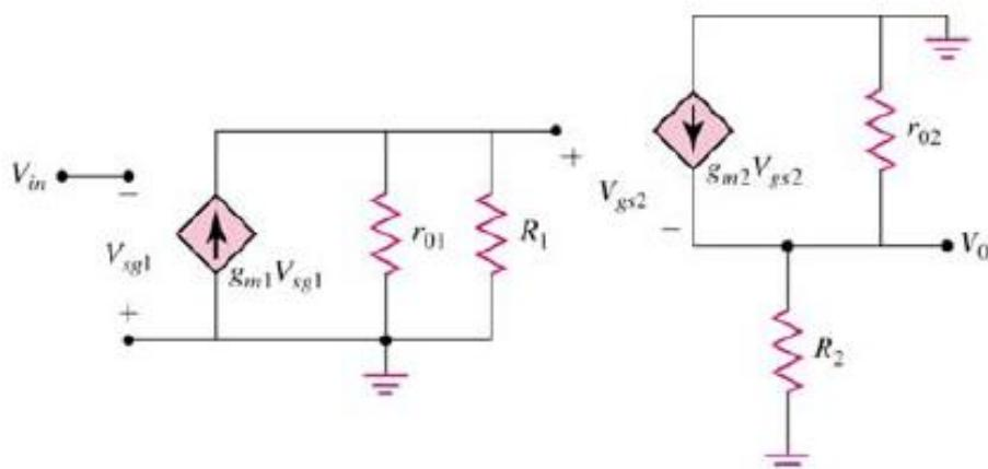
$$V_0 = (g_{m2} V_{sg2}) (R_2 \| r_{02})$$
