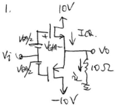
$$1^{\circ} \text{ for } V_0 = 5V, i_L = \frac{5}{10} = 0.5 A.$$
