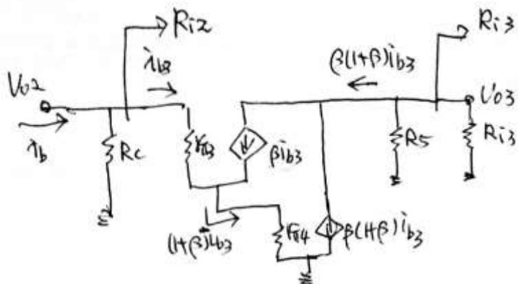
$$V_{o2} = i_{b3} \cdot (R_{i3} + (1 + \beta) R_{\pi 4}) = i_{b3} \cdot R_{i2}$$
