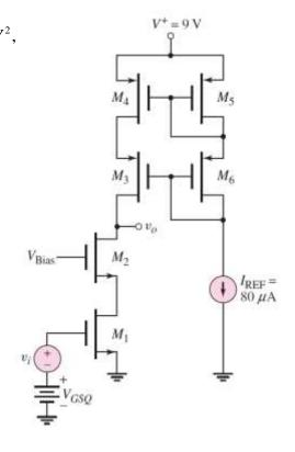
2. (25%) Assume that both transistors are biased in the saturation region, and that  $g_{m1} = g_{m2} = g_m$  and  $r_{o1} = r_{o2} = r_o$ . Suppose  $g_m \gg 1/r_o$ , show that  $R_o = \frac{2 + g_m r_o}{g_m (1 + g_m r_o)} \approx \frac{1}{g_m}$ .
