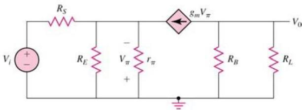
$$V_o = -g_m V_\pi (R_B \parallel R_L)$$
