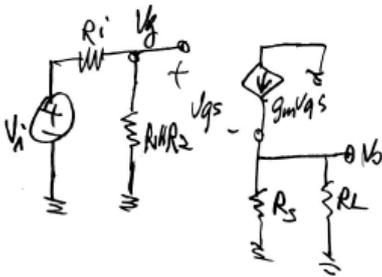
$$V_g = \frac{R_1 \parallel R_2}{R_1 \parallel R_2 + R_i} \cdot V_i$$
