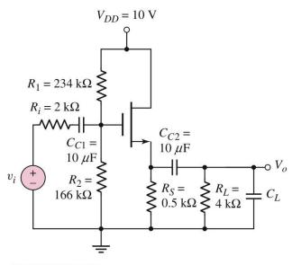
Copyright © The McGraw-Hill Companies, Inc. Permission required for reproduction or display 3. (30%) The transistor parameters are  $\beta=120, V_{BE(\text{on})}=0.7\text{V}, V_A=\infty, C_\mu=3\text{pF}$ , and  $f_T=250\text{MHz}$ . Determine the lower and upper corner 3dB frequencies.
