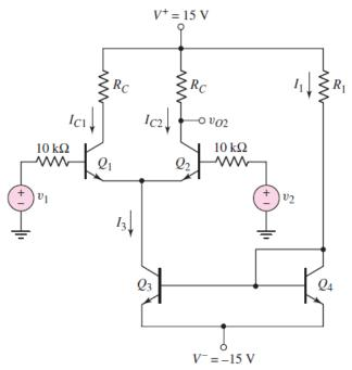
4. (25%) Assume that the parameters of the transistors are  $K_n = 0.2mA/V^2$ ,  $V_{TN} = 2V$ , and  $\lambda = 0.02V^{-1}$ . Determine the differential-mode voltage gain  $A_d = v_{O3}/v_d$ , where  $v_d = v_1 - v_2$ .
