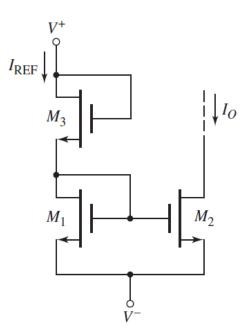
3. (25%) The parameters of the transistors are  $V_{TN} = 0.6$  V,  $V_{TP} = -0.6$  V,  $k'_n = 100\mu$ A/V<sup>2</sup>,  $k'_p = 60\mu$ A/V<sup>2</sup>, and  $\lambda_n = \lambda_p = 0.02$ V<sup>-1</sup>. The width-to-length ratios are shown in the figure. The value of  $V_{GSQ}$  is such that  $I_{D1} = 100\mu$ A, and  $M_1$  and  $M_2$  are biased in the saturation region. Determine the small-signal voltage gain  $A_v = v_o/v_i$ .
