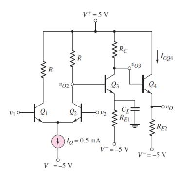
4. (25%) The circuit parameters are V<sup>+</sup>= 3 V, V<sup>-</sup>= -3 V, and  $I_Q=0.4m$ A. The NPN transistor parameters are  $\beta=180, V_{BE}(\text{on})=0.7\text{V}$ , and  $V_{AN}=120\text{V}$ , and the PNP transistor parameters are  $\beta=120, V_{BE}(\text{on})=0.7\text{V}$ , and  $V_{AP}=80\text{V}$ . Determine the one-sided differential-mode gain  $A_{d2}=v_{O2}/v_d$ .
